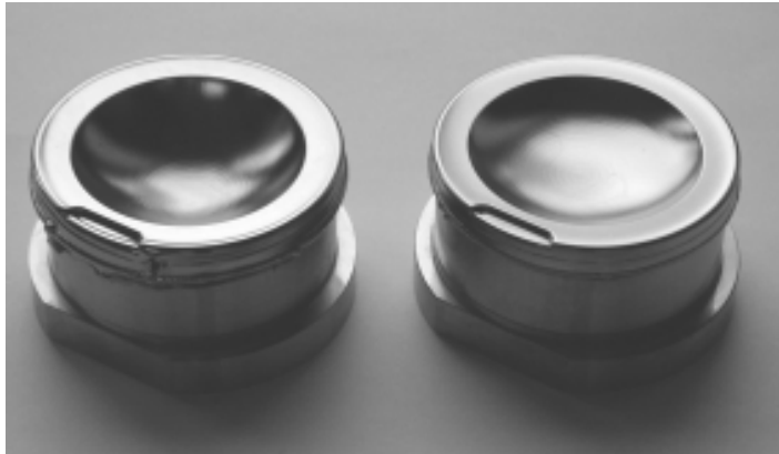
Micro-injection molding tools electroplated with a Nickel-Phosphorus layer before machining
